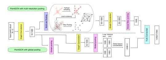
Fig. 1. Overall architecture for graph-CNN based point cloud classification model PointGCN. The top branch is the model architecture using multi-resolution pooling and the bottom branch is the model architecture using merely the global pooling layer.
